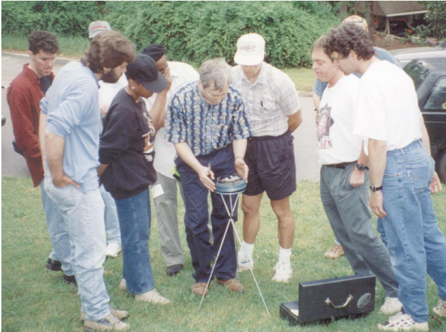
Above: Chris Carter shows students how to operate a Solar Pathfinder. The Solar Pathfinder is the tool for finding the best location for photovoltaic arrays and solar heat collectors.
